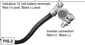
4.1.2. The power source must be capable of providing between 10.5V and 15.0V and able to supply the necessary current to operate the load.
